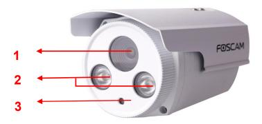
1 LENS: CMOS sensor with fixed focus lens
